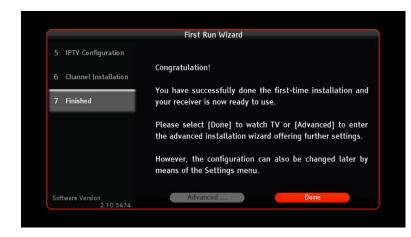
**Done** is shown. Press **OK**, to complete the initial installation.
