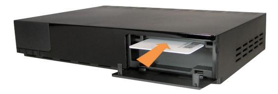
Insert the CONAX smartcard into the card reader with the gold chip facing forward. The chip must face downwards. Insert the card until it stops.
